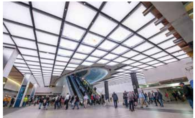
Above: MTA recently opened a section of its Penn Station Concourse project, which is widening the 33rd Street concourse from 30 feet to 57 feet and raising the ceilings to 18 feet.
